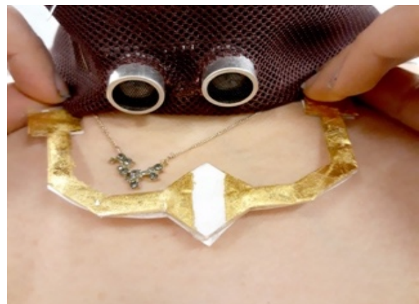
Figure 2: Gold necklace with a vibration motor, activated from sonar emission.
